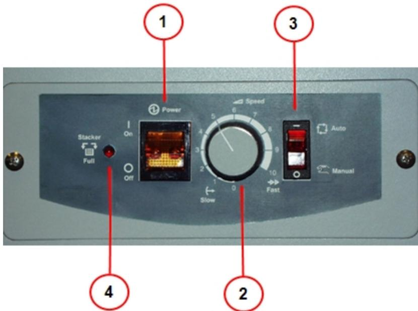
1. **Power Switch** - This is a rocker switch with indicator light. Press the top in to turn the Stacker on. Press the bottom in to it turn off.
