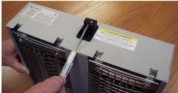
3. Remove blown fuse and insert replacement fuse, making sure it is the same type and rating.
