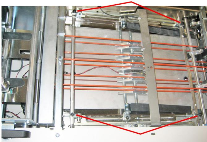
**Lock Screws on Accumulator Sides**
