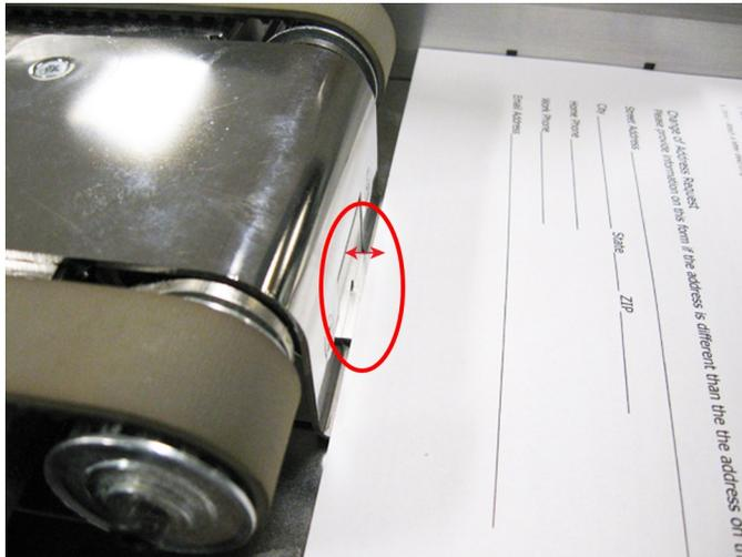
**1 to 2 mm Gap Between Material and Separator**
