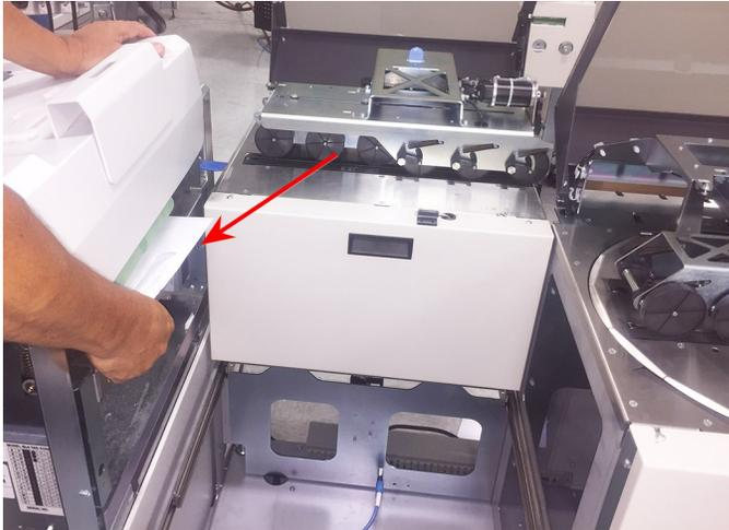
4. If the jam is inside the inserter:
