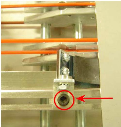
**Accumulator Strap Lock Screw (two screws, only one visible here)**
