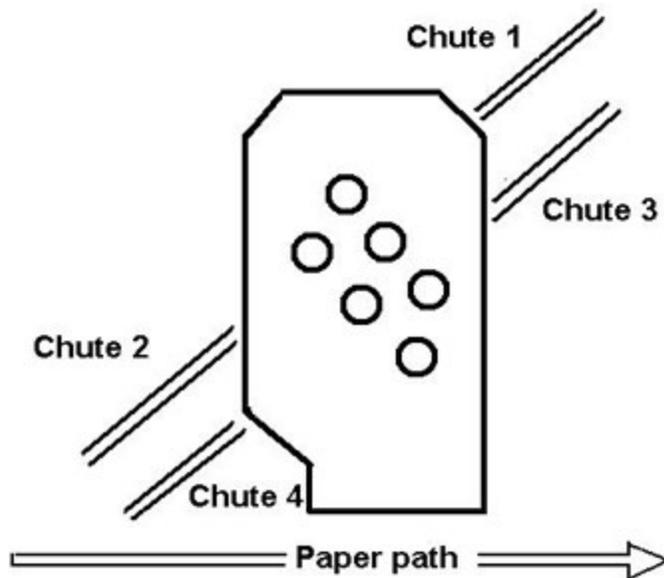
You can only access the auto buckle chutes by opening the folder and side access covers. These covers are interlocked, so the machine stops when the covers are open and will not restart until you close them.
