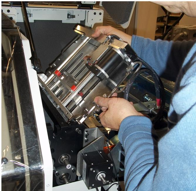
2. Lay the chute down on a flat surface, holding it firmly with one hand while using the other hand to remove the jammed material.
