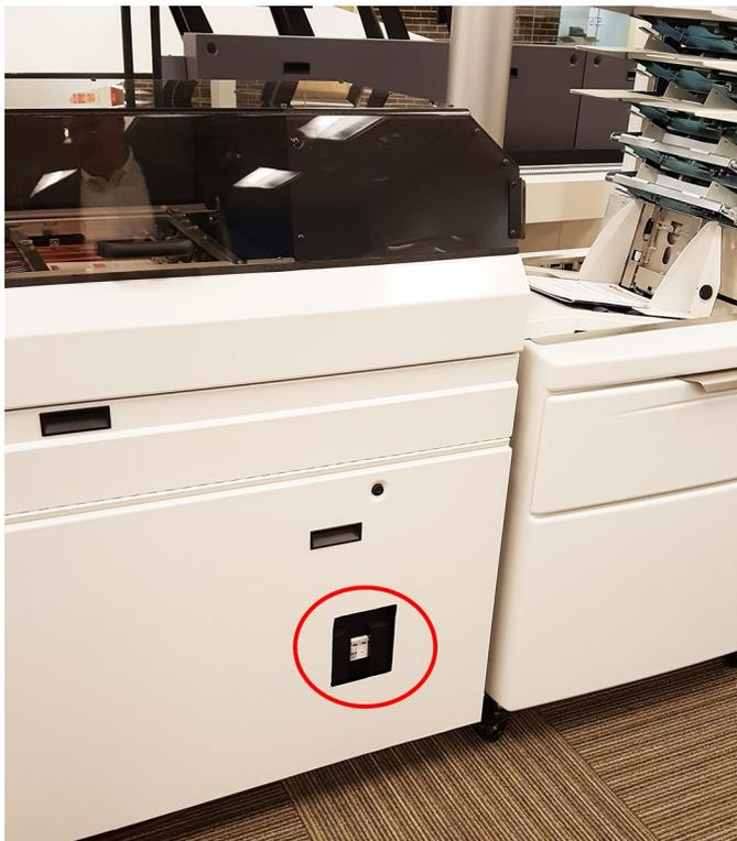
**Power Switch on the Pulse Input**
