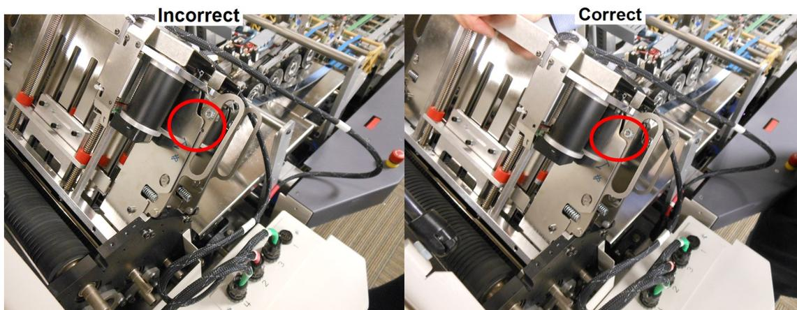
**Latch NOT Engaged (incorrect) and Latch FULLY Engaged (correct)**
