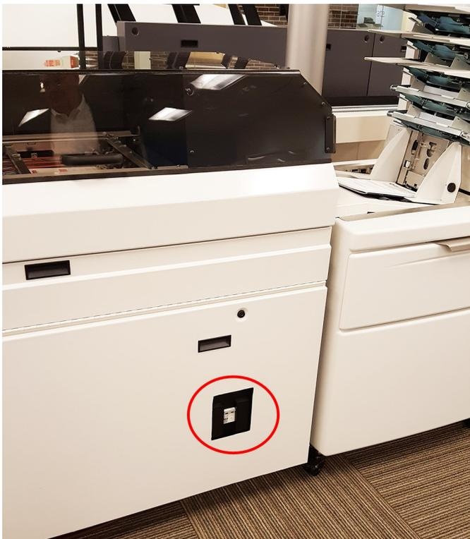
**Power Switch on the Pulse Input**
