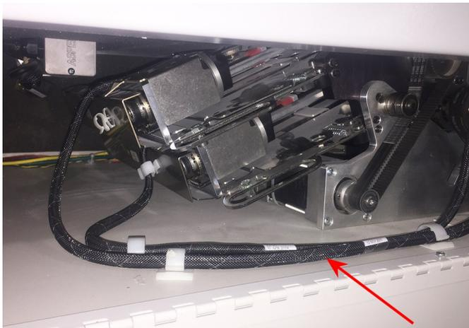
3. Pull out on the latch handles on auto buckle chute #4 and pull the chute back. (*Wiggle the chute slightly from side to side to disengage the latches on the sides of the chute from the folder; this allows you to pull the chute out.*)
