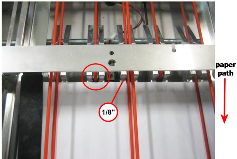
**Accumulator Ramp - Trail Edge 1/8" away from flat edge of ramp**
