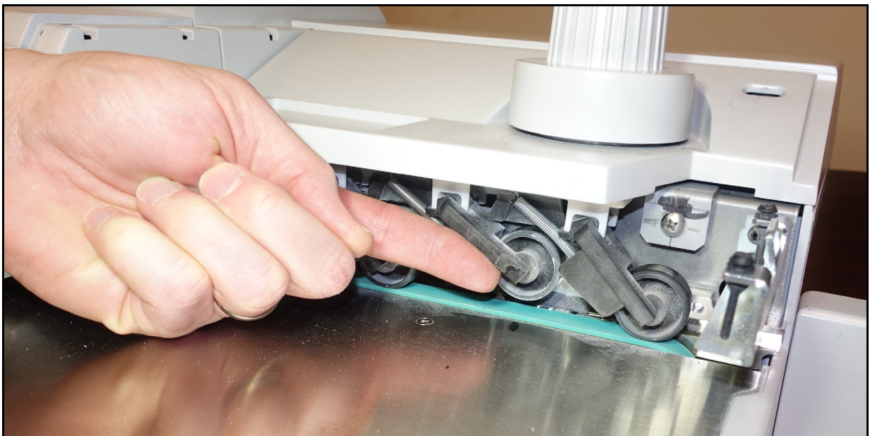
Figure 4-12: Cleaning under the nip wheels
