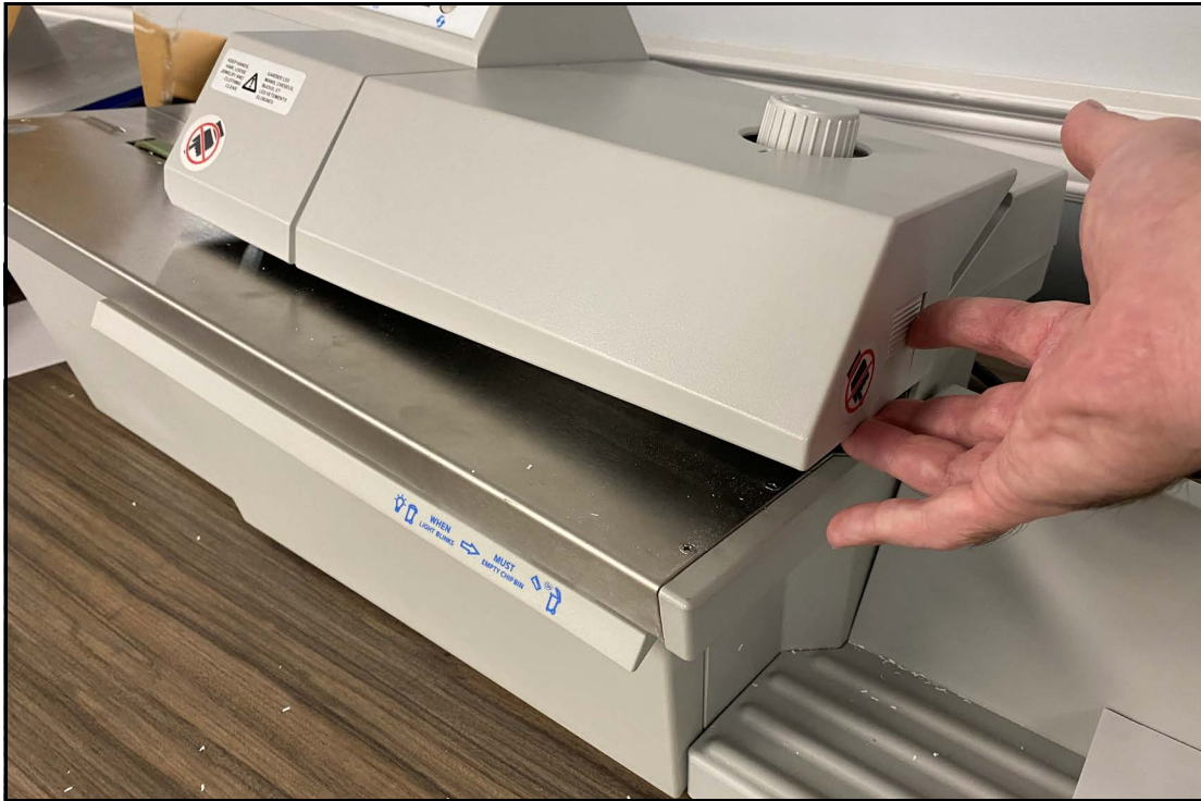
Figure 2-8: Top cover removal interlock triggering
