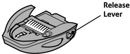
9. Slide the moistener back onto the machine. You should hear a click as it engages.
