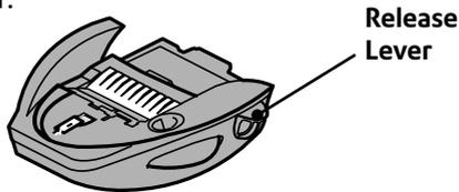
6. Slide the moistener back onto the machine. You should hear a click as it engages.
