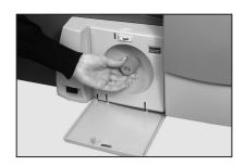
The Manual Advance Knob is located behind the drop down cover at the left front of the machine.
