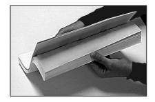
Jog the stack back into alignment. The Sheet Feeders take the paper stack aligned in a similar way to a photocopier paper cassette.
