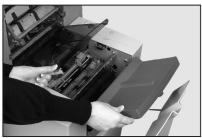
3. Squeeze together the two blue tabs (A) and lift the blue tab (B) to gain access to the sealer unit felts.
