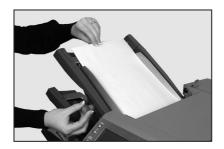
Take the stack of paper and aerate it to ensure the individual sheets are not stuck together.
