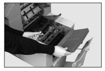
Points arrowed in the illustration can be unlatched to allow access to stalled material.
