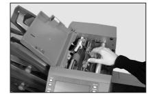
together and pivot the guide assembly back to its closed position. Release the two blue handles making sure the assembly is securely latched into position.
