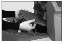
to release them. Slide the plate into its location guides and release the catches to lock the plate in position.
