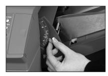
4. Set the blue separator shield lever to the **letter** required.
