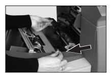
Push the rollers firmly down until they latch into position.
