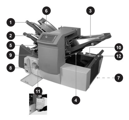
Sheet Feeder 1 This feeder is intended for feeding material that requires folding.
