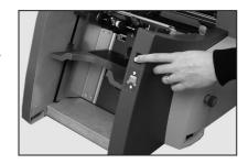
Adjust the side guides to the width of the envelopes being fed using the Side Guide Adjustment Knob, then backoff 1/4 of a turn.
