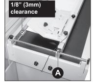
Adjust the side guide to give a clearance of about 1/8" (3mm) and retighten the front and rear end side guide knobs.
