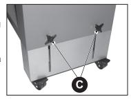
Position the stacker against the output end of the Inserter, centered with the output. Make sure the stacker is positioned firmly against the Inserter covers.
