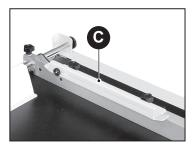
5. The Inserter exit deflector must be fully raised.
