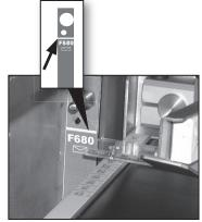
If necessary, loosen the height adjustment knobs (**C**) on each leg in turn and readjust the stacker height.
