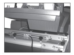
The exit roller bridge (A) should already have been installed to the Inserter output.
