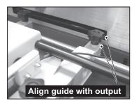
If necessary, loosen the height adjustment knobs (**A**) on each leg in turn and readjust the stacker height.
