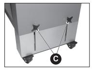
Position the stacker as close to the Inserter output as possible and centered with the output. When positioned correctly, lock all four castors.
