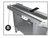
Check the stacker alignment. The top of the side guide should fit into the cut-out on the exit roller bridge assembly.
