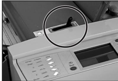
Adjust the Side Guide to the width of the sheets being fed, using the Side Guide Adjustment Knob, then back-off a 1/4 of a turn. This will set the correct clearance between the guides and the material.
