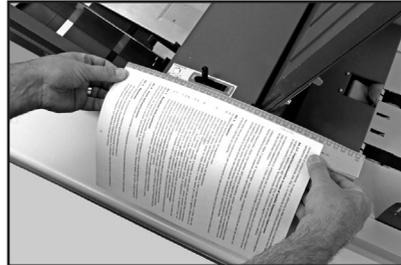
Select a relevant preset length (i.e. US Letter/ A4) by screen key or select Custom and then press the +/- keys until the length of your paper (in millimetres) is displayed. When the paper length is correct, press **OK...**
