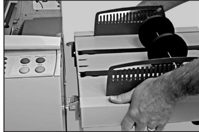
It is fitted to the machine with two hooks which slide into the apertures at the exit of the machine.
