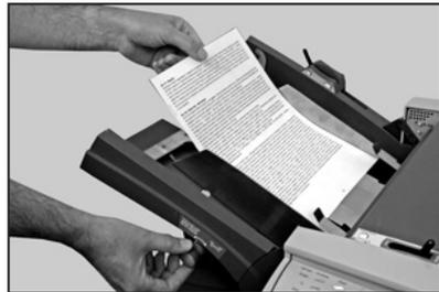
**Note:** When using manual feed the material weight should not exceed 5 sheets of 80gsm or a total weight of 400gsm. The machine speed is automatically limited to Level 1 for ease of use when running a manual feed job.
