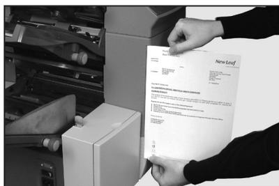
Press **Change (+/-)** until the length of your paper (in millimeters) displays.
