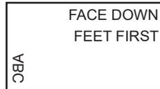
5. Place the paper stack onto the feed deck. Allow the deck to move down and the top of the paper stack to slide under the feed roller.
