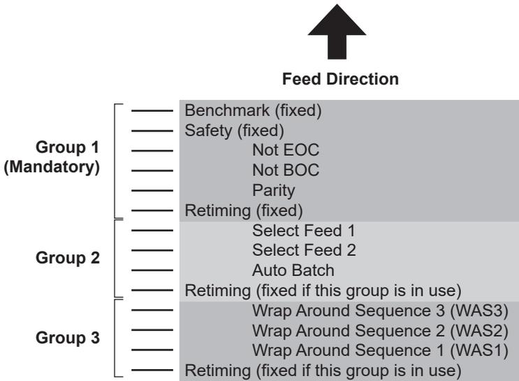
Print sheets in reverse collation order. In this way, the last sheet processed in each set is the address sheet and the first sheet processed is the last of each set.
