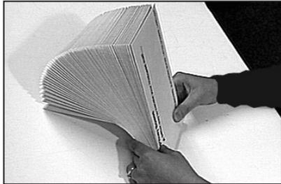
**IMPORTANT !** Check that lead edge of the first envelope is under the front feed roller and that the stack of envelopes is shingled on the deck as shown.
