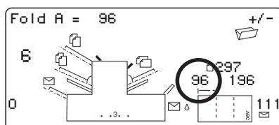
If you want to change the standard setting, press **Change (+/-)** until the length of the fold required is displayed. The symbol | — | shows the fold panel you are adjusting.
