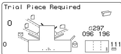
If you have material loaded, press **Trial Piece**. The machine sets itself and runs a test piece for you to check.
