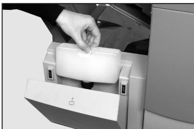
**Note:** If the sealer unit has emptied completely, allow enough time for the solution to soak through the sealer mechanism. This helps assure good seals.
