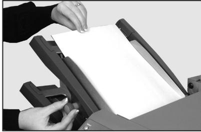
2. Take the stack of paper and aerate it to ensure that individual sheets are not stuck together.
