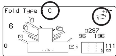
**Note:** For OMR scanning jobs, DO NOT manually change the fold length dimensions for Fold A and Fold B. These are set automatically by the machine.
