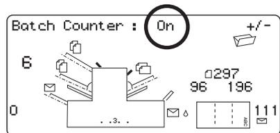
If the batch counter is turned on, the machine will now request the batch quantity. The default quantity is 50, but you may select any value up to 999 using the **Change (+/-)** buttons.
