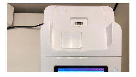
2. Fix the blanking plate on the device where the scale was located.
