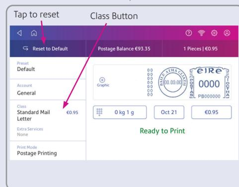
The **Class** button shows the current Class selected. Tap the **Class** button to enter the Class screen.
