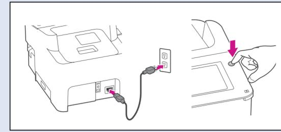
Connect your device to a power source and turn on the power switch.
