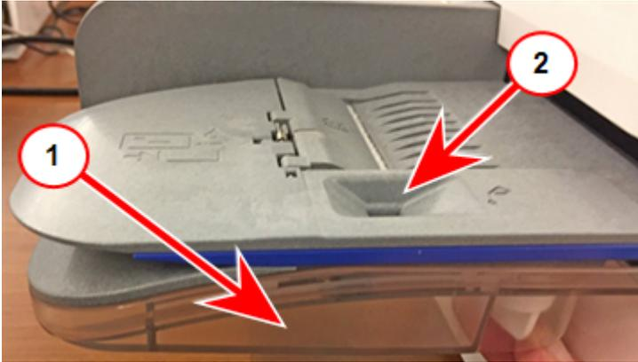
2. Add enough E-Z Seal® to bring the sealant level up to the bottom of the fill hole **(2)**. Do not overfill the tank.
