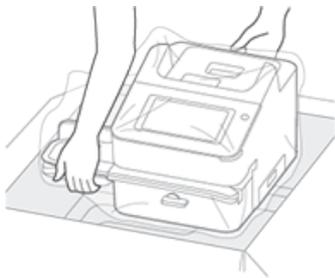
2. **Important:** Be sure to grab hold of the entire feeder, not just the moistener flap when lifting the device out of the box.
