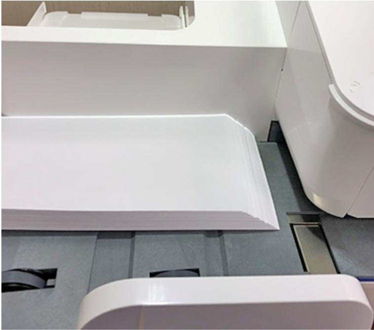
3. Slide the side guide up to the mail stack. Leave about 1/8" space (about the thickness of 2 quarters) between the stack and the side guide so the envelopes do not drag against the guide.
