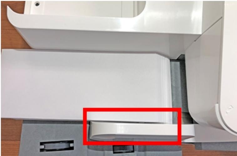
4. Push the stack into the feeder until you feel resistance. The image shows how far into the feeder you need to position the stack. The side guide is pulled away to show the edge of the envelopes.
