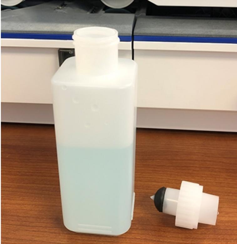
5. Screw the cap back on and place the bottle back in its original site (upside down in the device).
