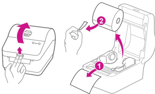
3. Install the label roll and feed the label through the media guide.
